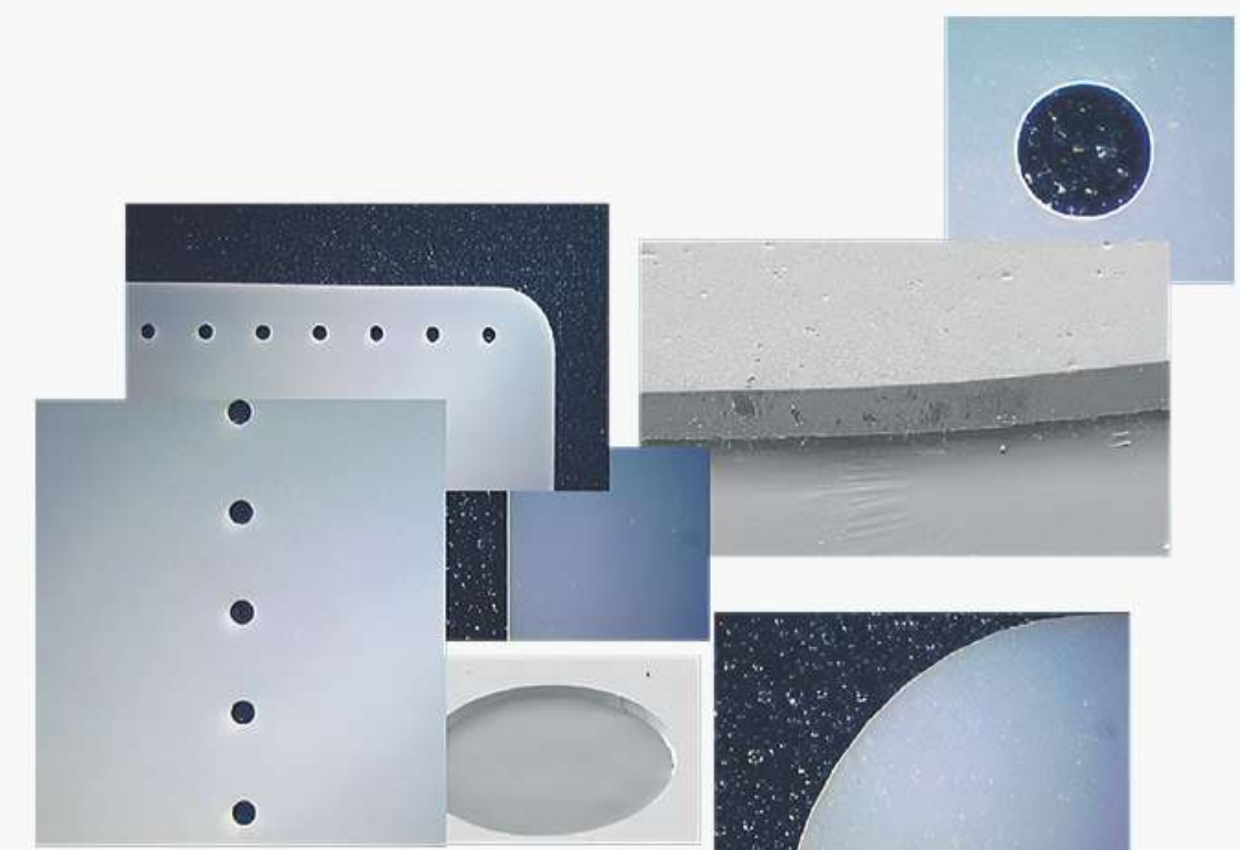
Laser cut features in Thin E-Strate®
