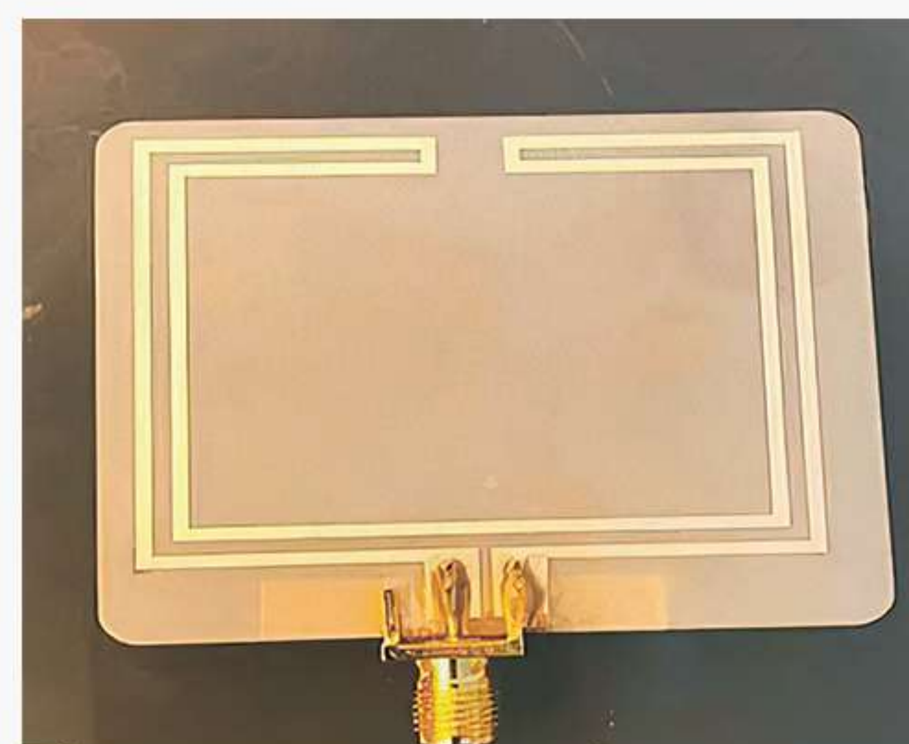
Printed silver folded-dipole antenna
