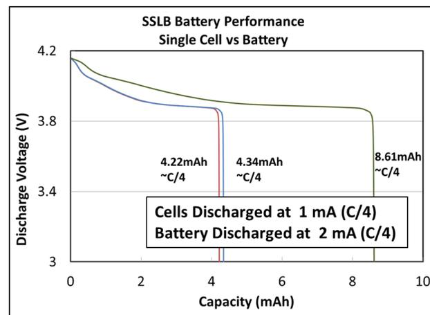
**Figure 4.** SSLB battery capacity scales with the number of cells in the stack.
