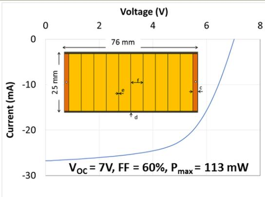
**Figure 8. CdTe mini-modules on YSZ achieved ~7% efficiency. Based on recent small cells with 11% efficiency, module efficiencies approaching 20% should be possible with further optimization.**
