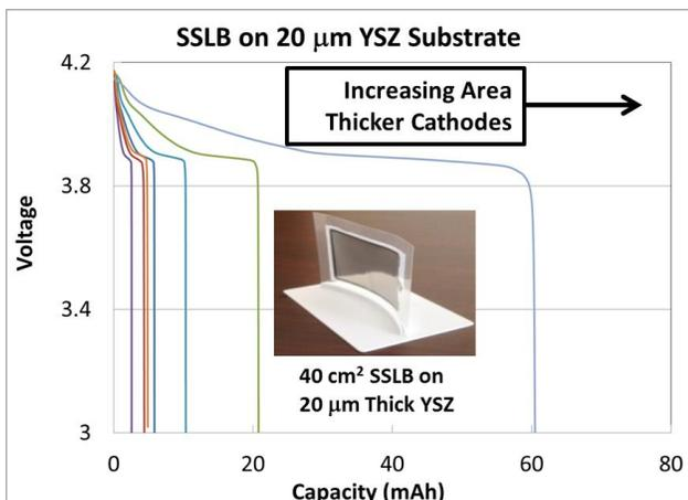
**Figure 3.** SSLB cells, deposited on 20  $\mu\text{m}$  thick YSZ, have capacity that increases linearly with area and cathode thickness; inset is a large area SSLB.
