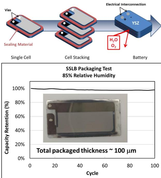
**Figure 2.** SSLB packaging employs YSZ as both the substrate and hermetic packaging with edge sealing adhesives between layers (top). SSLB with thickness <math><100\ \mu\text{m}</math> shows stable cycling in high humidity.
