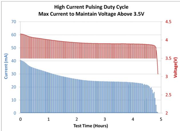
**Figure 5. The low SSLB internal resistance supports repeated high current pulses over the entire discharge; in this case 40 mA pulses (10C) at the beginning of life and ~25 mA on average (6C).**
